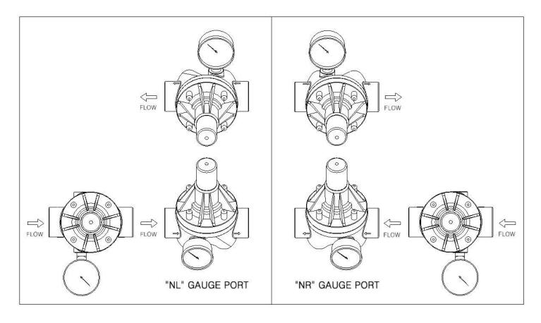
The gauge is always placed on the intake side of the back-pressure valve. If your system configuration matches one of the three options on the left, then -NL is the product code to use on your PO. If your system configuration matches one of the three options on the right, then -NR is the product code to use on your PO.
